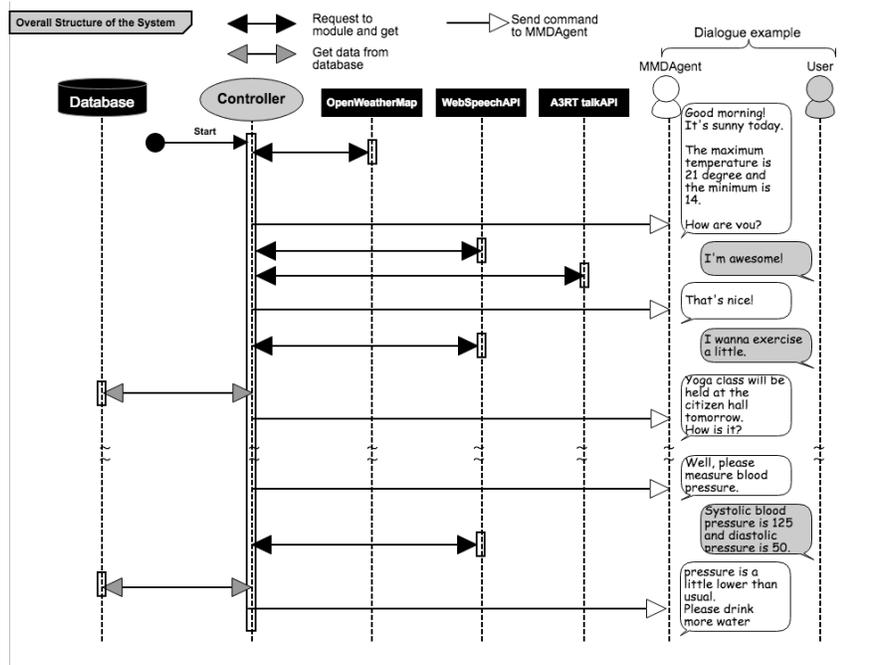
Fig. 1 Processing flow of the system and an example of the dialog
